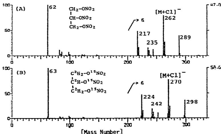
Fig. 1. NICI mass spectra of (A) GTN and (B)  $[\text{}^2\text{H}_5, \text{}^{15}\text{N}_3]\text{GTN}$  with dichloromethane as reagent gas.
