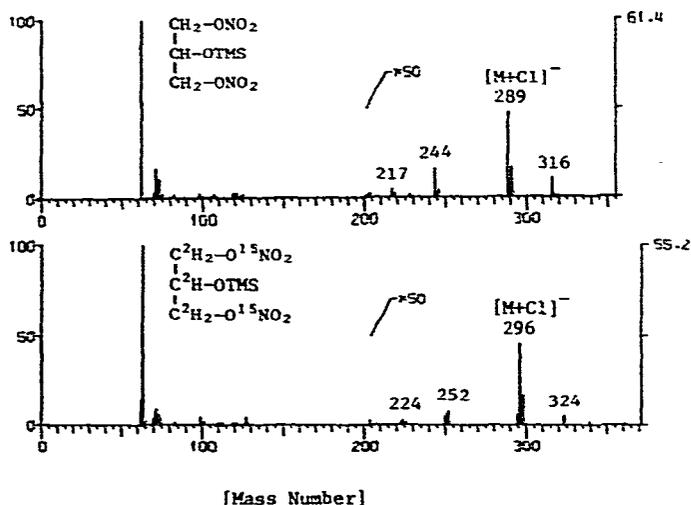
Fig. 3. NICI mass spectra of (A) 1,3-GDN and (B) 1,3-[<sup>2</sup>H<sub>5</sub>, <sup>15</sup>N<sub>2</sub>]GDN with dichloromethane as reagent gas.
