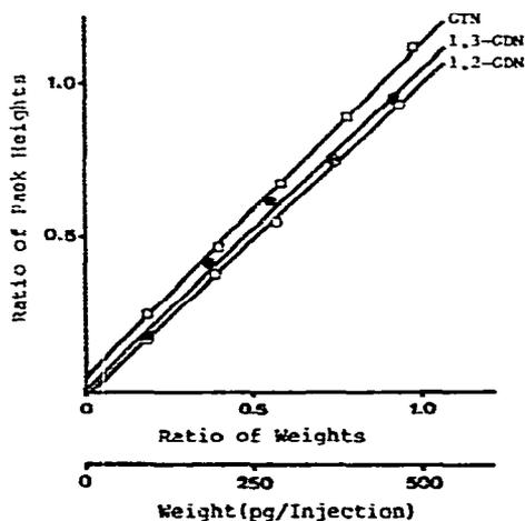
Fig. 4. Calibration graphs for GTN, 1,2-GDN and 1,3-GDN.
